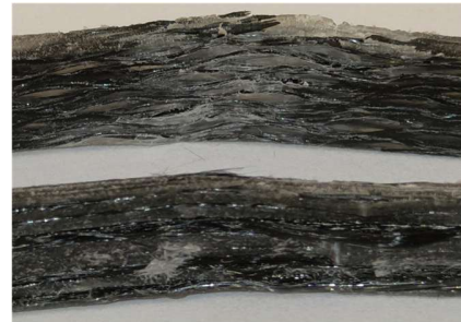
FIGURE 16: THE BENDING FRACTURES OF SPECIMENS OF PREPREG FIBER ON THE TOP AND DRY FIBER WITH IN-SITU IMPREGNATION ON THE BOTTOM
