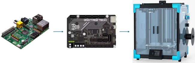
FIGURE 1: DATA FLOW MODIFICATION TO AN ENDER 6 COMMERCIAL MEX PRINTER
