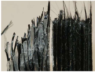
FIGURE 14: THE TENSILE FRACTURES OF SPECIMENS OF PREPREG FIBER ON THE LEFT AND DRY FIBER WITH IN-SITU IMPREGNATION ON THE RIGHT
