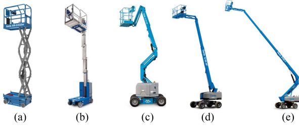
Fig. 2. (a) Scissor lift, (b) vertical mast lift, (c) articulating lift, (d) telescopic lift, and (e) telescopic articulating lift [8].
